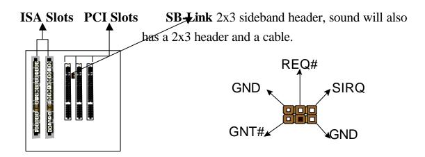
Note: The default on-board Forte Media sound is recommended. After installing the sound driver, the user can enable this function without plugging any cable into jumper of SB-Link.
