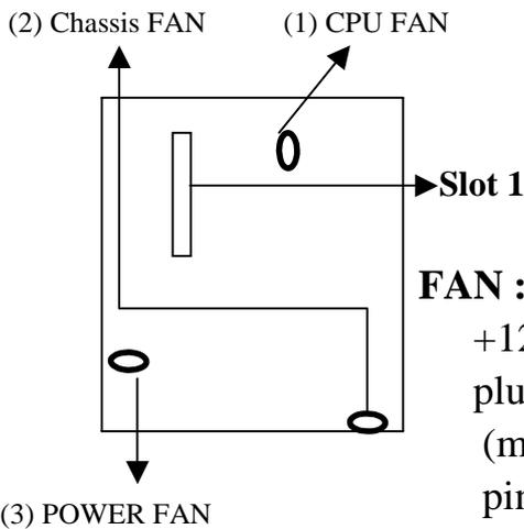
**FAN : CPU cooling fan connector.** Wire with +12V voltage (most likely red wire) must be plugged into pin2, and GROUND wires (most likely black wire) must be plugged into pin3. Please confirm the wire color re-presentation with your supplier.
