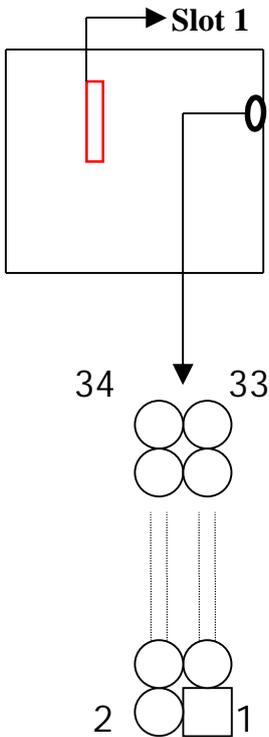
**FDC1 : this connector is used to connect the floppy drive through a cable.**
