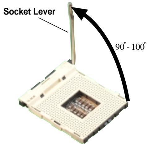
3. Position the CPU above the socket such that its marked corner matches the base of the socket lever.
