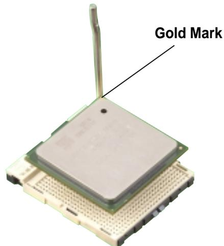
5. When the CPU is in place, push down the socket lever to secure the CPU. The lever clicks on the side tab to indicate that it is locked.
