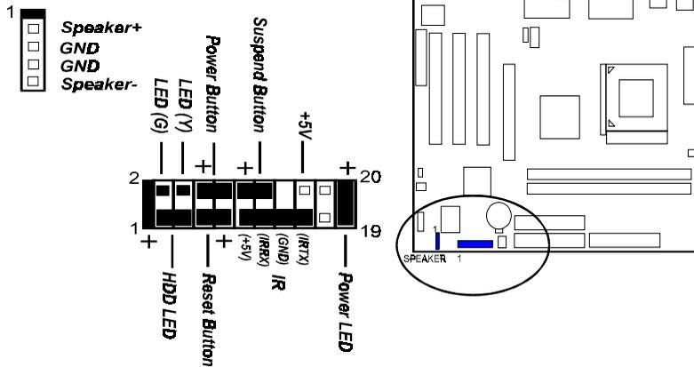
**Power LED** is connected with the system power indicator to indicate whether the system is on/off. It will blink when the system enters suspend mode.
