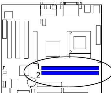
Press the clips with both hands to remove the DIMM.
