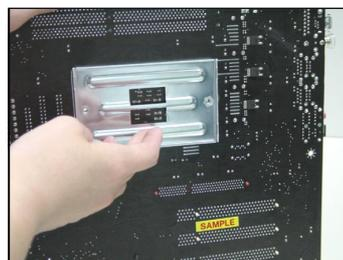
3. Turn over the mainboard again, and place the mainboard on the flat surface. Locate the two screw holes of the mainboard.
