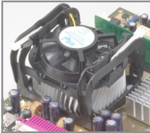
4. Connect the CPU fan cable. With the fan, heatsink, and the retention mechanism in place, attach the CPU fan cable to the connector on the motherboard labelled CPUFAN
