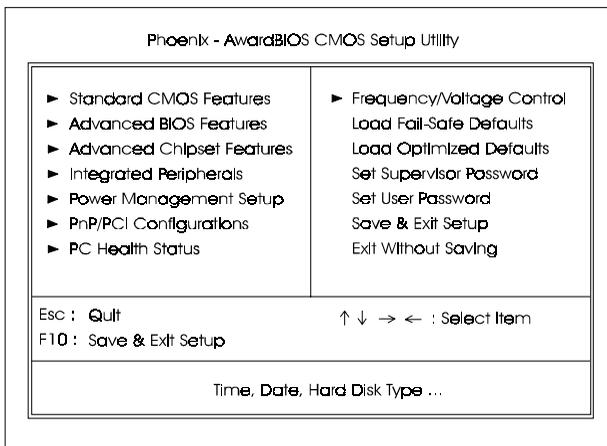
The Setup utility program allows updates to the mainboard configuration settings. The BIOS setup values will be saved in the CMOS. It is executed when the user changes system configuration; user changes system backup battery; or the system detects a configuration error and asks the user to run the Setup program. Use the arrow keys to select and press **Enter** to run the selected program.
