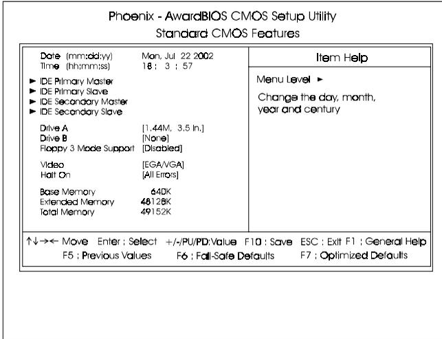
The Standard CMOS Setup screen is displayed above. Each item may have one or more option settings. The system BIOS automatically detects memory size, thus no changes are necessary. Use the arrow keys to highlight the item and then use **PgUp** or **PgDn** keys to select the value you want in each item.
