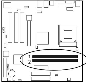
Press the clips with both hands to remove the memory module.
