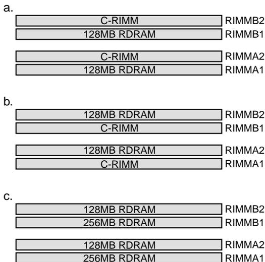
**NOTE:** When using only two memory modules, it is recommended that you use configuration a.
