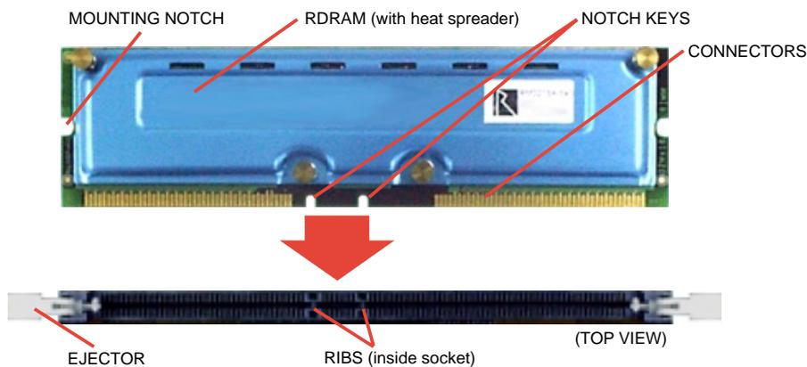
2. With the ejectors in the open position (as shown), push down gently but firmly on the memory module until it snaps into place. The guides on the socket's ejectors should go through the two mounting notches on the module and the ejectors should close. If necessary, push the ejectors inward to secure the module in place.
