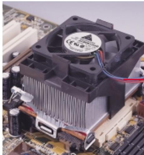
Connect to the CPU fan connector.
