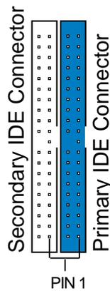
**NOTE:** Orient the red markings (usually zigzag) on the IDE ribbon cable to PIN 1.
