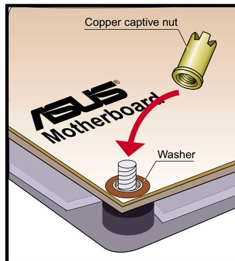
**IMPORTANT:** This step is a MUST! The washers are necessary to prevent shorting.
