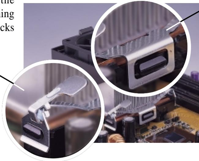
**WARNING!** Be sure that there is sufficient air circulation across the processor's heatsink by regularly checking that your CPU fan is working. Without sufficient circulation, the processor could overheat and damage both the processor and the motherboard. You may install an auxiliary fan, if necessary.
