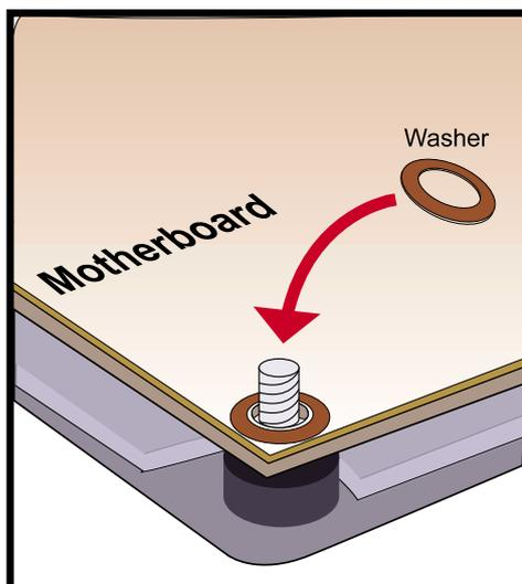
Tighten the four copper captive nuts over the washers.
