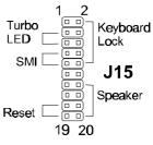
**Pins [17 & 19] Reset switch lead** - Connects to the Reset Switch lead from the system case. The reset switch is used to "cold-boot" the system without actually turning off the power, reducing wear and tear on the power supply.
