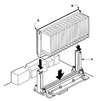
The CPU Heatsink may not appear as shown in the illustrations. Your heatsink will most likely be fitted with an electric fan, connect the fan connector to the Header on the motherboard marked for this purpose.
