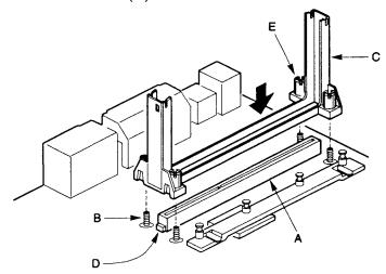
2. To position the mechanism (C), orient it as shown above. The tab (D) on the connector fits into a notch in the base of the mechanism. When properly seated, the base of the mechanism is flush with the motherboard.
