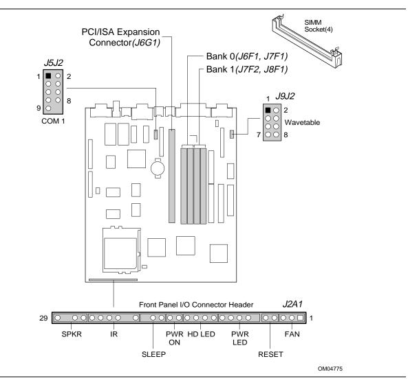
Figure 3. Motherboard Connector Locations
