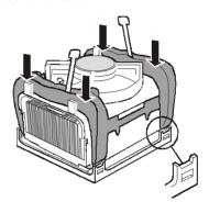
2. Hold the Fan/Heatsink steady and press one of the clip assembly's locking levers down into the locked position.
