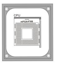
Heatsink/fan assembly mounting frame
