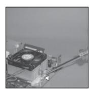
Press the retention clip over the socket lug with a flathead screwdriver
