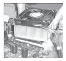
Position the heatsink evenly on the CPU so that one edge hangs over, but does not contact the socket
