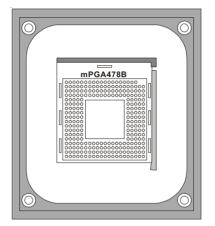
Fan/Heatsink assembly retention mechanism
