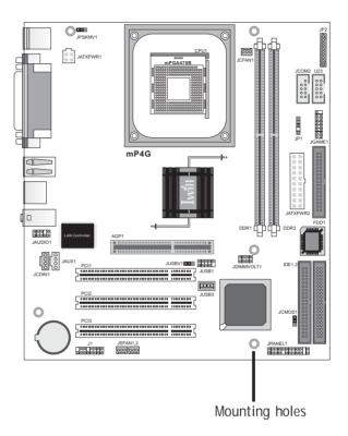
5. Attach the board to the housing by inserting mounting screws in all the holes and tightening them snugly.
