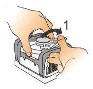
3. Repeat the process for the second clip. Keep holding the Fan/Heatsink steady so that you don't damage the TIM. The locking levers should now hold the heatsink securely in the Retention Mechanism.
