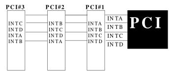
Figure 7: The Combination of PCI INT#lines
