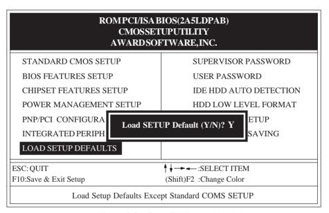
Figure 3-8 LOAD SETUP DEFAULT
