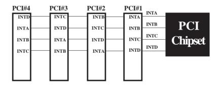
Figure 3-7 The Combination of PCI INT# lines
