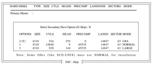
Figure 8: IDE HDD Auto Detection
