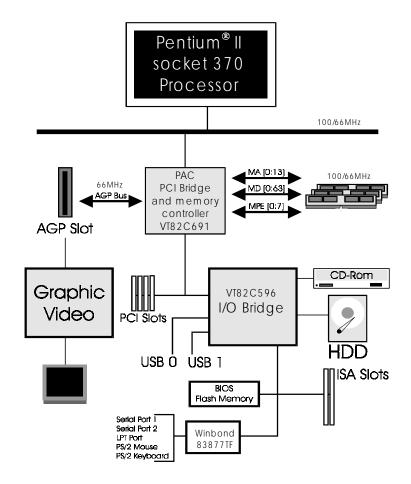
Figure 5: System Block Diagram
