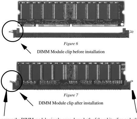
To remove the DIMM module simply press down both of the white clips on both sides and the module will be released from the socket.
