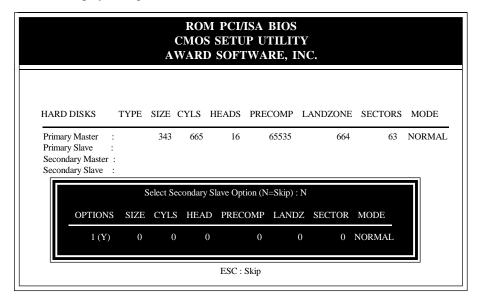
Figure 3-9 IDE HDD AUTO DETECTION
