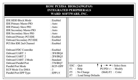
Note: If you don't use the Onboard IDE connector, than use On-card (PCI or ISA card) IDE connector. You will set Onboard Primary PCI IDE: Disabled and Onboard Secondary PCI IDE: Disabled from CHIPSET FEATURES SETUP UTILITY. The Onboard PCI IDE cable should be equal to or less than 18 inches (45 cm.).
