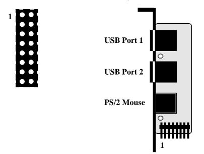
Figure 4-1 USB Port & PS/2 Mouse Adapter
