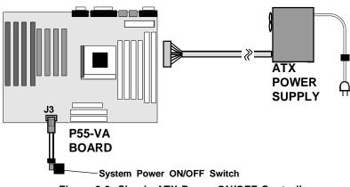
Figure 3-3: Simple ATX Power ON/OFF Controller
