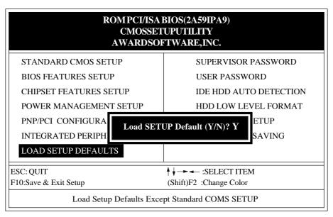
Figure 4-8 LOAD SETUP DEFAULT
