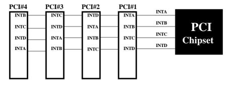
Figure 4-7 The Combination of PCI INT# lines
