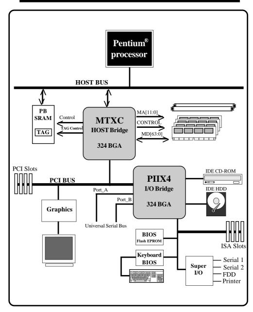
Figure 1-2 System Block Diagram
