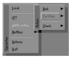
In which **Disk** indicates hard disk options **Partition** indicates partition options **Check** indicates check options
