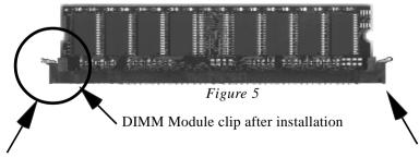
To remove the DIMM module simply press down both of the white clips on either side and the module will be released from the socket.
