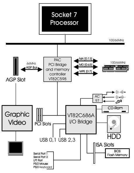
Figure 5: System Block Diagram
