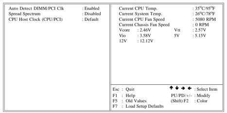
Figure 9: Sensor And CPU Speed Setup
