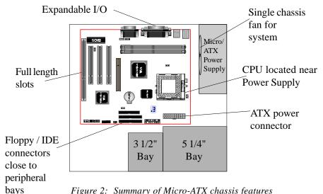
Figure 2: Summary of Micro-ATX chassis features
