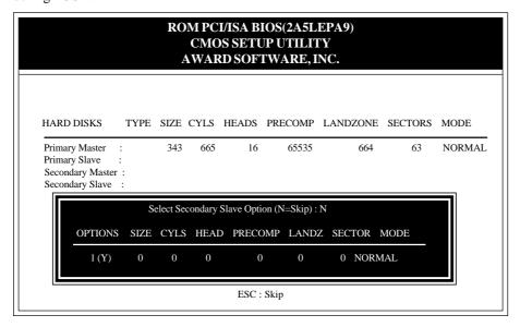
**Figure 3-9 IDE HDD AUTO DETECTION**
