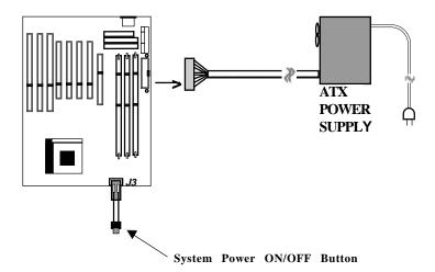
Figure 2-2: Simple ATX Power ON/OFF Controller
