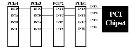
Figure 3-7 The Combination of PCI INT#lines
