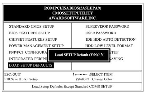
Figure 3-8 LOAD SETUP DEFAULT
