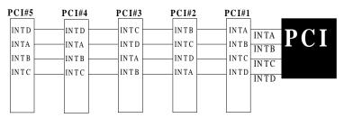
Figure 7: The Combination of PCI INT#lines
