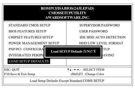
Figure 3-8 LOAD SETUP DEFAULT
