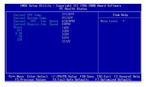
**Current CPU Temperature**: This is the current temperature of the CPU.
