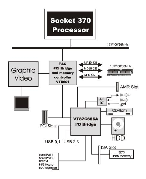
Figure 5: System Block Diagram
