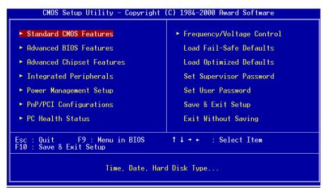
Figure 1: CMOS Setup Utility
