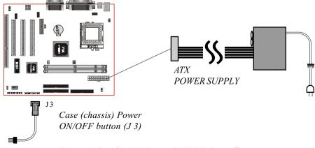
Figure 4: Simple ATX Power ON/OFF Controller
