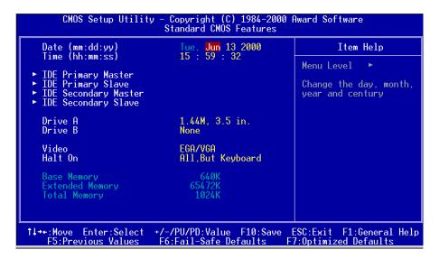
Figure 2: Standard CMOS Setup
