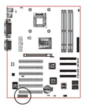
**CNR Conn.:** The board supports one CNR connector to provide a Modem Code (MC) or Phone-line base networking and 10/100 Ethernet base networking configuration.
