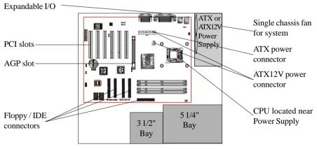
Figure 2: Summary of ATX or ATX12V chassis features
