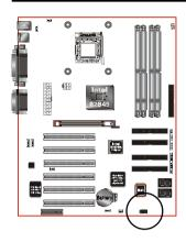
**USBCON1:** USB port header pins for share with two USB ports.
