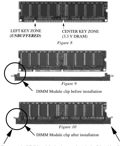
To remove the DIMM module simply press down both of the white clips on either side and the module will be released from the socket.
