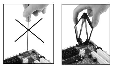
The BIOS socket may be damaged if using an improper method to replace the BIOS chip.
