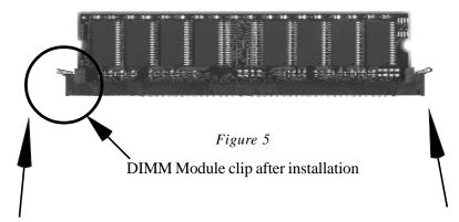
To remove the DIMM module simply press down both of the white clips on either side and the module will be released from the socket.
