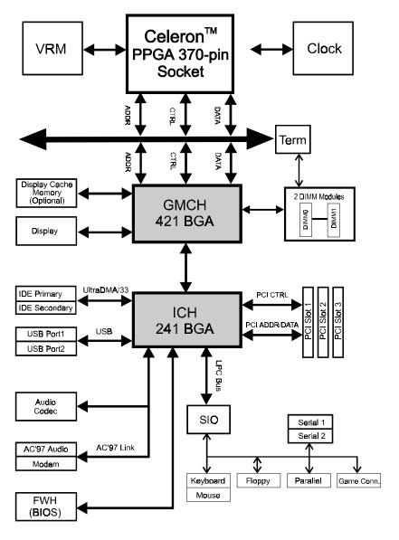
Figure 5: System Block Diagram
