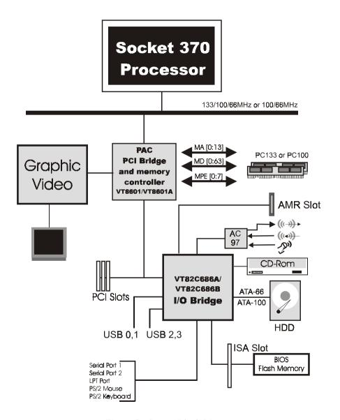
Figure 5: System Block Diagram
