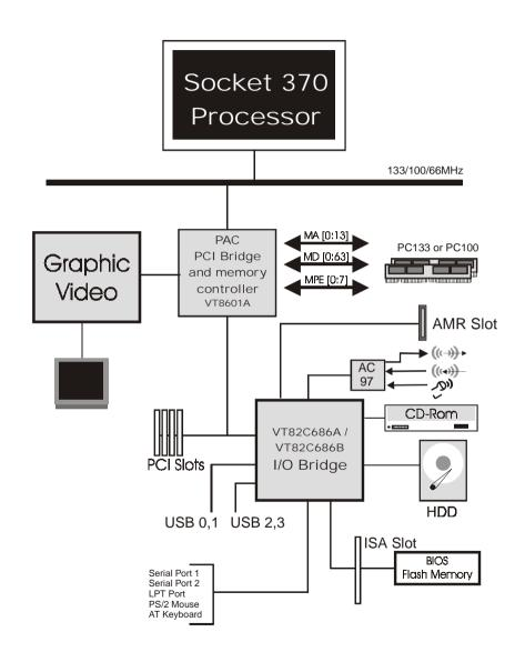
Figure 3: System Block Diagram
