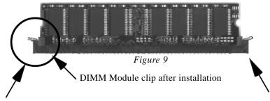
To remove the DIMM module simply press down both of the white clips on either side and the module will be released from the socket.
