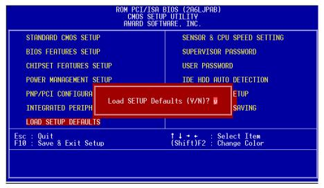
Figure 7: Load Setup Defaults
