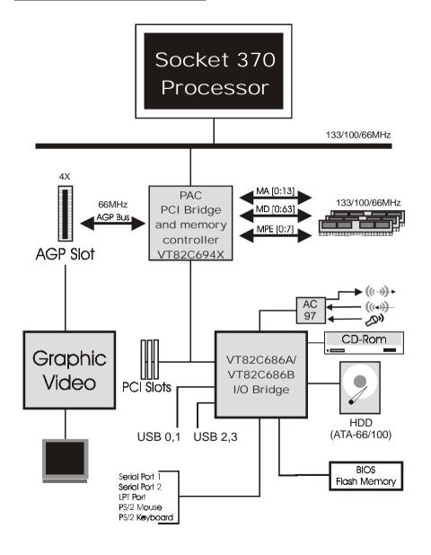
Figure 5: System Block Diagram
