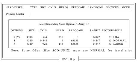
Figure 8: IDE HDD Auto Detection
