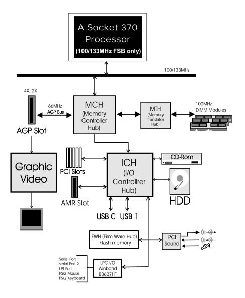
Figure 6: System Block Diagram
