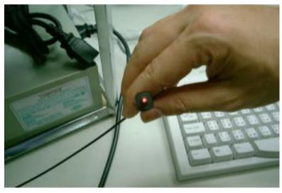
Please note that signal beam may cause severe damage to the eyes. For your safety, please point the output end to a piece of white paper to check if thebeam is in function.
