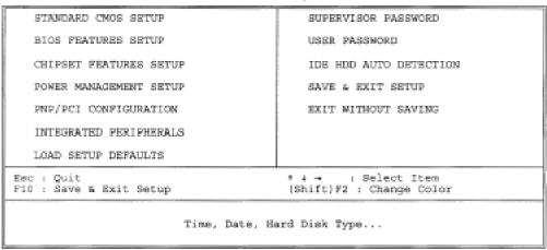
Figure 1: CMOS Setup Utility
