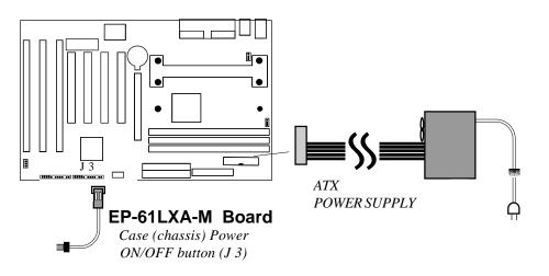
Figure 4: Simple ATX Power ON/OFF Controller
