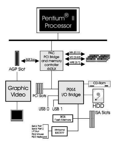
Figure 5: System Block Diagram
