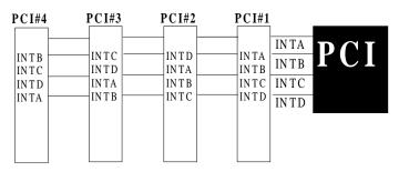
Figure 7: The Combination of PCI INT#lines
