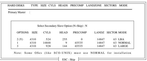
Figure 8: IDE HDD Auto Detection
