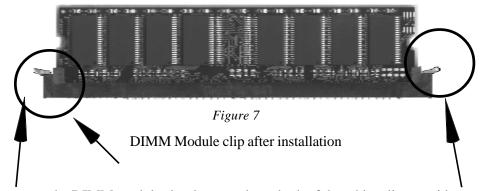
To remove the DIMM module simply press down both of the white clips on either side and the module will be released from the socket.
