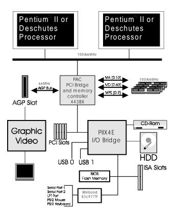
Figure 5: System Block Diagram
