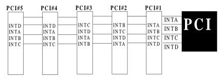
Figure 7: The Combination of PCI INT#lines
