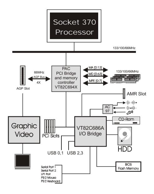
Figure 5: System Block Diagram
