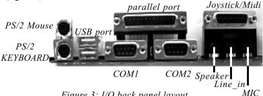
Figure 3: I/O back panel layout
