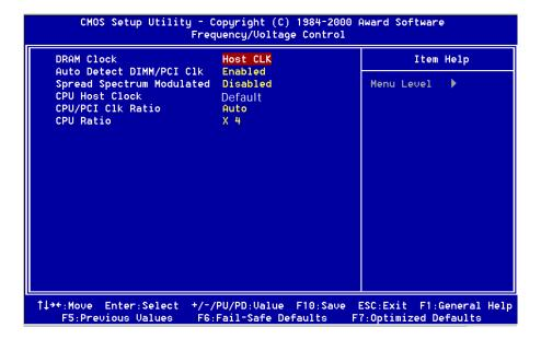
**DRAM Clock:** The item will synchronize/asynchronize DRAM operation clock. *Host Clock:* DRAM has same working clock with CPU host bus.
