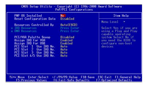
Figure 7: PCI Configuration Setup
