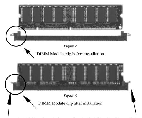
To remove the DIMM module simply press down both of the white clips on either side and the module will be released from the socket.
