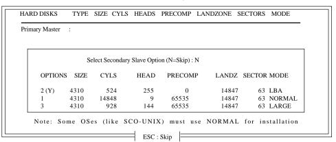
Figure 8: IDE HDD Auto Detection
