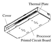
Figure 1: Pentium<sup>®</sup> II or Deschutes Processor CPU with S.E.C. Cartridge
