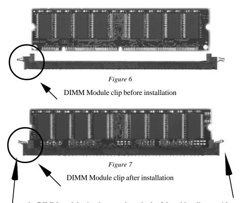
To remove the DIMM module simply press down both of the white clips on either side and the module will be released from the socket.
