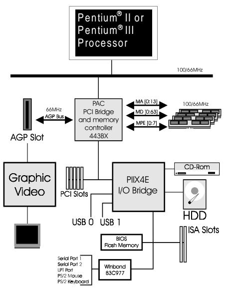
Figure 5: System Block Diagram
