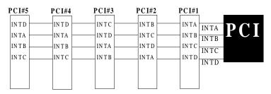
Figure 7: The Combination of PCI INT#lines
