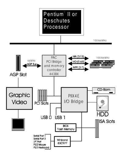
Figure 5: System Block Diagram
