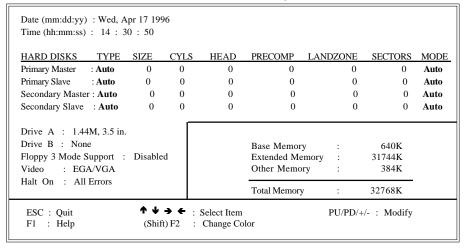
Figure 2: Standard CMOS Setup
