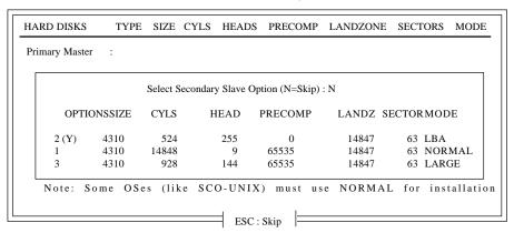
Figure 8: IDE HDD Auto Detection
