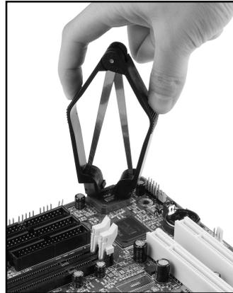
The BIOS socket may be damaged if using an improper method to replace the BIOS chip.
