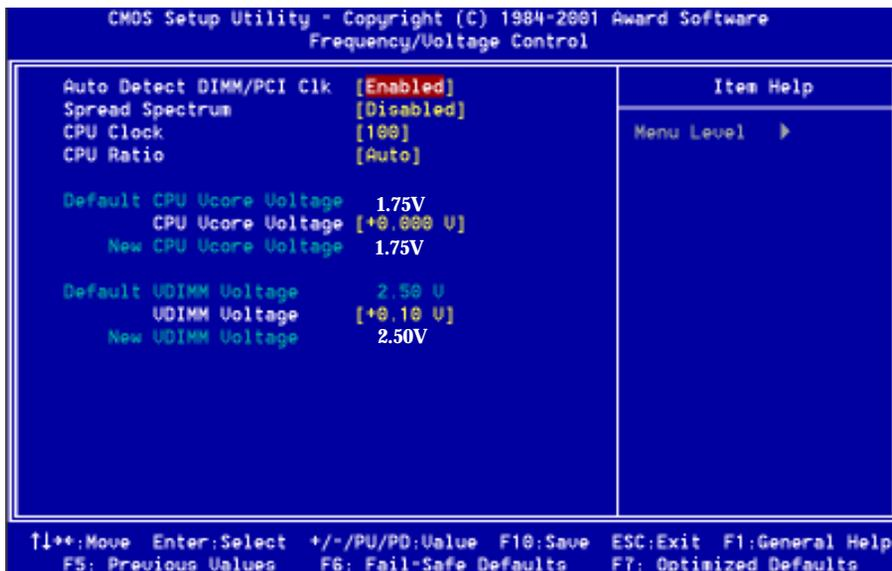
**Auto Detect DIMM/PCI Clk:** When enabled the motherboard will automatically disable the clock source for a DIMM socket which does not have a module in it. Same applies for PCI slots. This setting will reduce the EMI. The default is Enabled.
