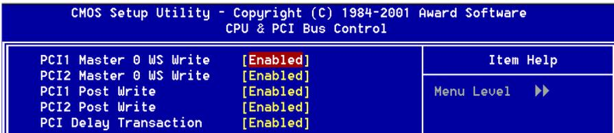
**PCI1/2 Master 0 WS Write:** When Enabled, Writes to the PCI bus are commanded with zero wait states.
