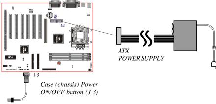
Figure 4: Simple ATX Power ON/OFF Controller
