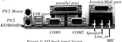
Figure 3: I/O back panel layout
