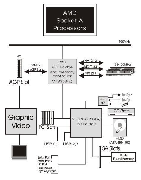
Figure 5: System Block Diagram
