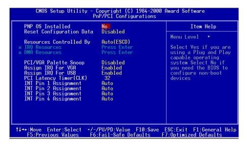
Figure 7: PCI Configuration Setup
