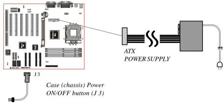
Figure 4: Simple ATX Power ON/OFF Controller
