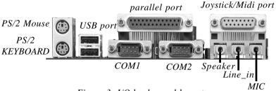
Figure 3: I/O back panel layout
