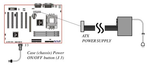
Figure 4: Simple ATX Power ON/OFF Controller
