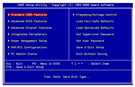
Figure 1: CMOS Setup Utility
