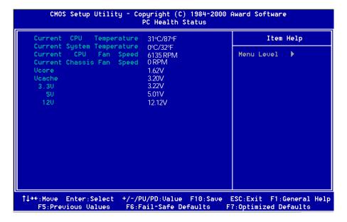
Current CPU Temperature: This is the current temperature of the CPU.
