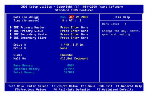
Figure 2: Standard CMOS Setup
