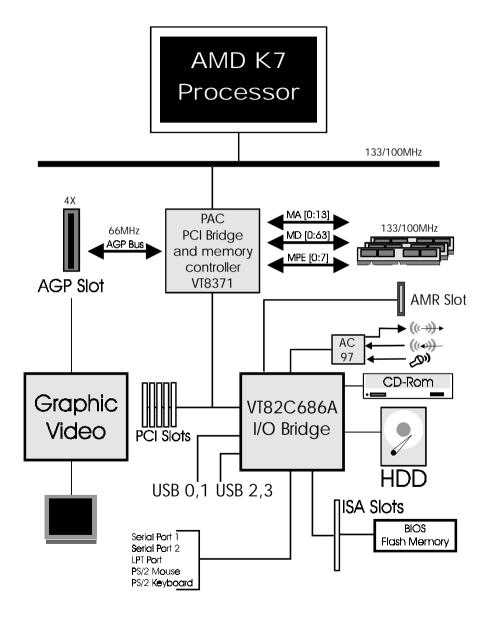
Figure 5: System Block Diagram
