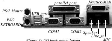
Figure 3: I/O back panel layout
