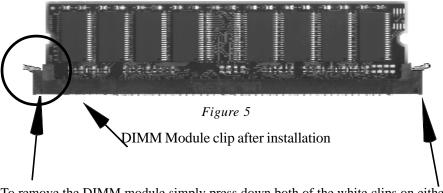
To remove the DIMM module simply press down both of the white clips on either side and the module will be released from the socket.
