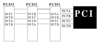
Figure 7: The Combination of PCI INT#lines
