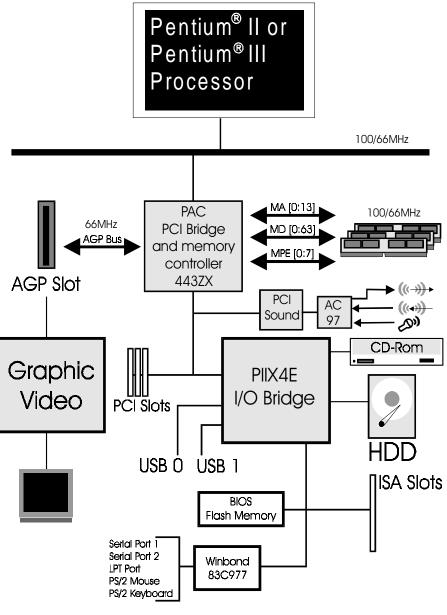
Figure 5: System Block Diagram
