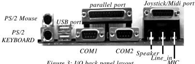
Figure 3: I/O back panel layout
