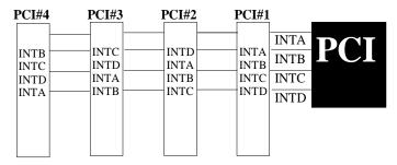
Figure 7: The Combination of PCI INT#lines
