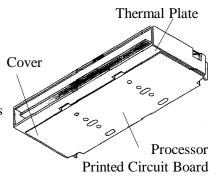
Figure 1: Pentium® II Processor CPU with S.E.C. Cartridge
